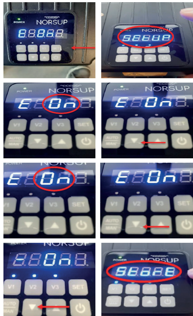
Fig. 11: Variable speed pump parameter setting steps
